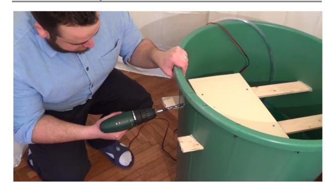
Place the device on the plywood board, and run its electric cable and the water pump's through the hole in the barrel.
