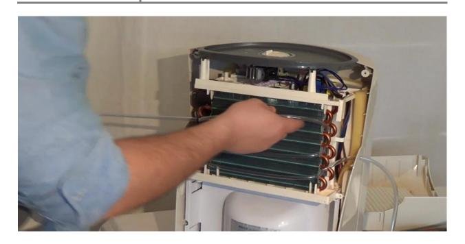
Be sure to test if the hose doesn't get in the way when trying to put the cover back on. And don't pull too hard on the hose when looping it, or it may get strangled and the water won't flow through it.
