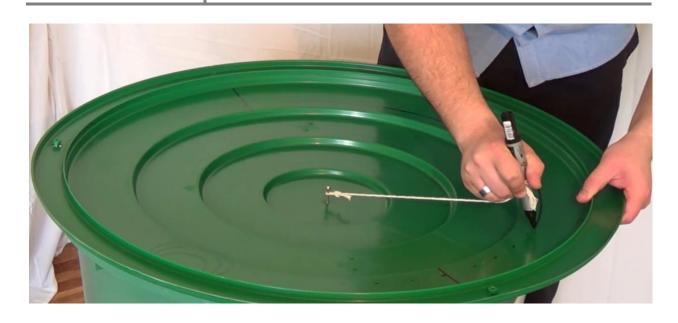
It's time to cut the barrel cap at the specified size. I used a box cutter knife because the cap was soft plastic. If the one provided with your barrel is harder, use a metal hacksaw to get the job done.
