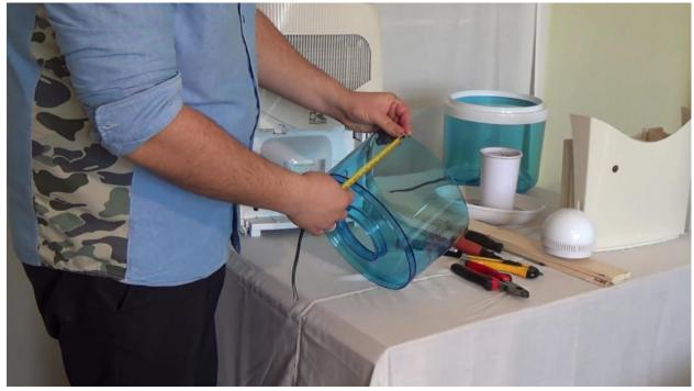
From the bottom of the holes you drilled earlier, mark 6 + 2 inches (or your own value + 2 inches) down towards the bottom. Do that 8 times inside around the barrel. Those 2 extra inches ensure that the wooden boards that will support the dehumidifier won't touch the top of the water filter container.
