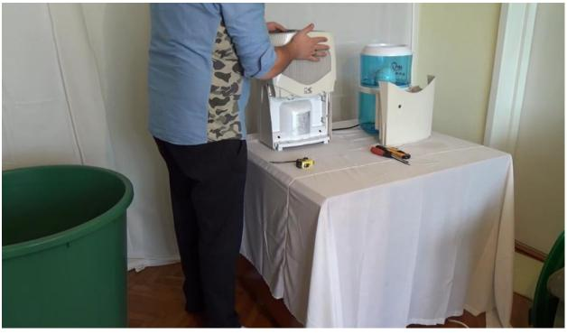
Measure the height from the base of the device to the condenser cover. You can go higher if you want. The important thing is that the dehumidifier's air intake and air exhaust (that's at the back) are above the measured level. I got 10 inches on mine.
