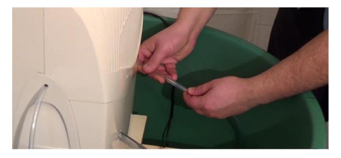
On the other side of the water cooling system, connect a hose that will lead to the tap. Use the same method as before. Cut the tap hose down to size.
