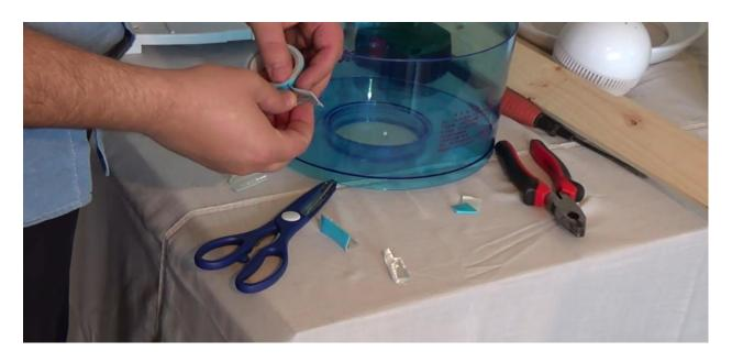
Make sure you place the protectors at the same level inside the barrel, so the previously cut cap will rest on all of them.
