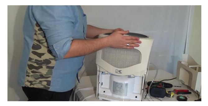
Now put the condenser cover back on. Be careful not to squeeze the water cooling hose.
