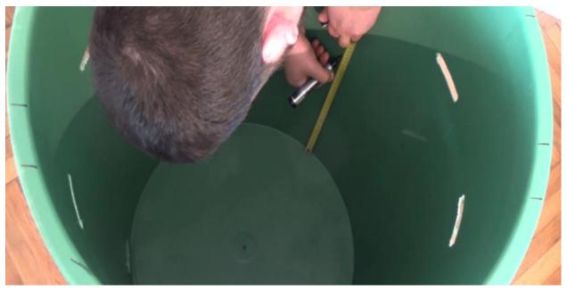
Measure the inside diameter at that level. We'll cut one of the barrel caps at that diameter to create the filtered water container. I got 1.9 ft.
