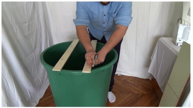
Now you'll have to drill holes in the barrel, so the wooden boards will go through it. That will create a stand for the dehumidifier.
