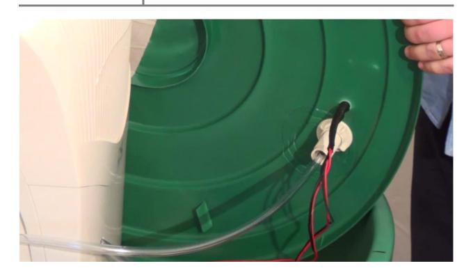
Put the barrel cap on the barrel. Be careful not to crack it, rip or strangle the hoses.
