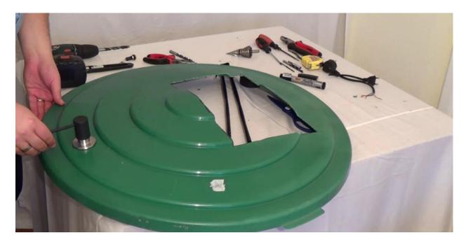
Pull the pump's extension cord through the hole drilled in the cap. You'll have to make the wire connections outside the cap. This of course depends on the type of power switch you choose. But for most of them you'll have to follow this method.
