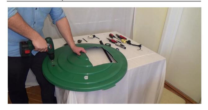
Mount the water tap on the barrel cap.
