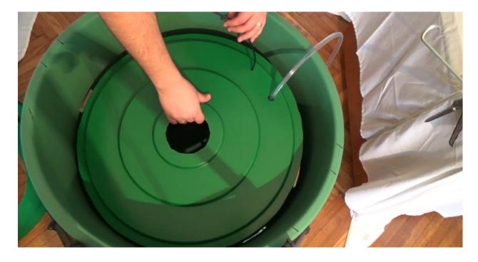
Place the cap on the silicone protectors. It should be nice and fit. If it's not, trim the cap a little with a pair of scissors.
