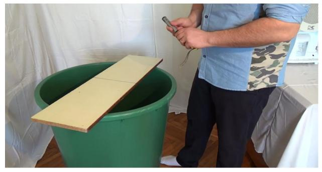
Next we'll cut the wooden board. You'll need 2 pieces with a length equal to the barrel top diameter. For me, that was 2 ft 3 inches long, 3 inches wide. The width of the wooden board should be anywhere between 2 and 3 inches, but not very thick.
