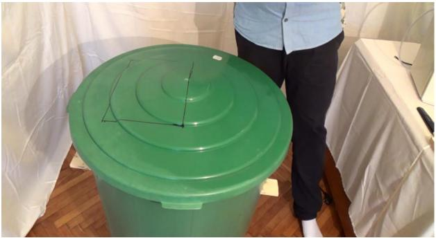
Use a box cutter knife or a metal hacksaw, depending on how hard the barrel cap is.
