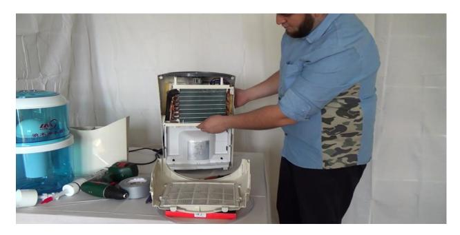
On the inside of the cover you'll see the air filter. Because we want to use the condensed water for drinking, we'll apply an auto cabin filter on the original. It will drastically improve the water quality and the lifespan of the water filter.
