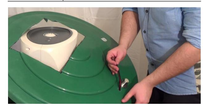
Pull the 2 wires from the extension apart, and cut one of them. Now connect one end of the previously cut wire to one of the switch's poles, and the other end to the second pole on the switch. Insulate them properly with insulating varnish, and push the switch in its hole.
