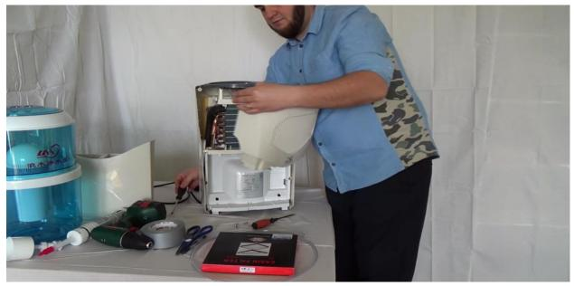
You will have to gain access to the air filter and the condenser behind it. The condenser is the cold circuit of the device. Because it's cold, it will condensate water from the surrounding air. And to be sure you found it, it looks like a car radiator, probably in two layers with a half inch gap between the two.
