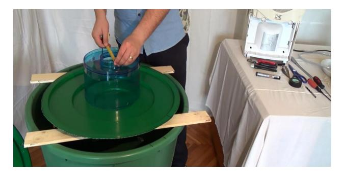
Give it a couple of radiuses, and use the divider like you did before and cut the round disc out.
