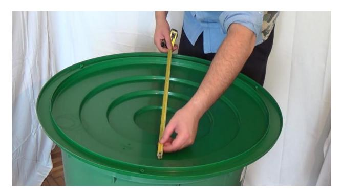
What I did is split the diameter in half to get the radius, and mark about 30 radiuses around the cap.
