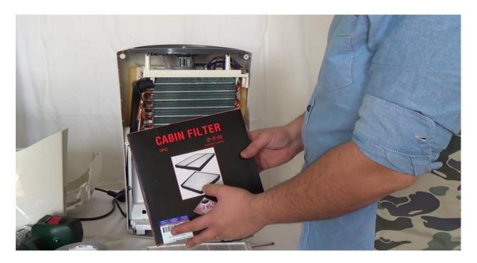
Measure the cabin filter and cut it down to size for a perfect fit. Use duct tape to bind the filters together just like you see in the video.
