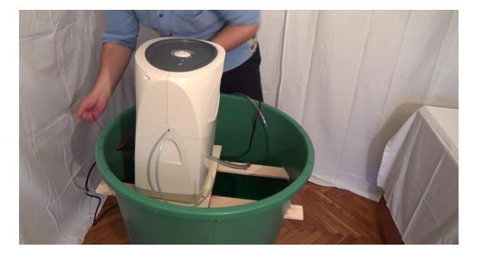
Place the water drain hose inside the water filter container. Cut it down to size if necessary so it won't bend.
