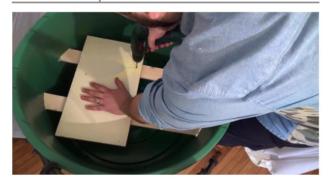
Use sanitary silicone to insulate and glue the 2 wood boards to the barrel.
