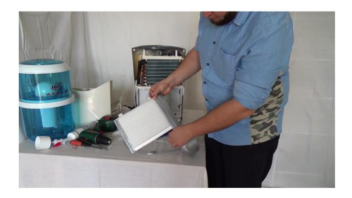
After you've finished taping the filter, put it back in its original position. In my case, it's the condenser cover.
