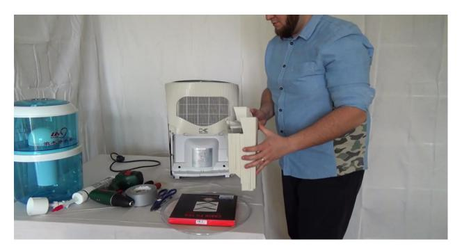
The condenser cover should be right above it and probably houses the air filter. I had to get through 6 screws to take it off.
