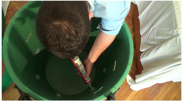
Now put some sanitary silicone on the bottom of the barrel, where the water pump will be placed.
