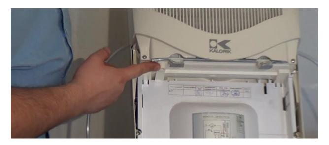
I couldn't find a hose for a perfect fit. So I had to widen it a little. I used the flame from a lighter to heat the tip of the hose. It will become malleable and you'll be able to force it on the water drain. Now drill a hole in the water tray, large enough for the hose to pass through it. When reattaching the water tray to the dehumidifier, proceed with caution so you won't pull the hose off the drain.
