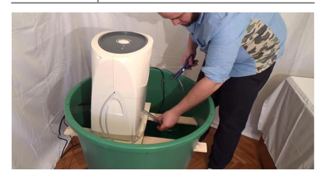
Cut the water pump hose so it won't be too long. The longer the circuit, the harder it will be to pump the water out. Connect it to one side of the water cooling hose. Mine didn't fit perfectly the first time. So I found a hose with intermediary size and used it as a reduction. It's important that it won't leak.
