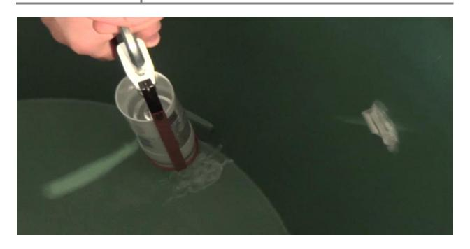
Put the water pump over it and press 'till it sticks to the bottom. This way, when you'll have to move the system, the pump will stay firmly set in its position.
